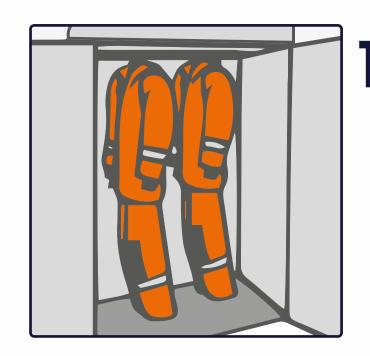
It's a good idea to hang the parts of your work outfit on the same hanger. Begin by hanging the trousers, and then hang the jacket. Then slide in the hanger onto the proper opening in the ceiling of the drying cabinet.
